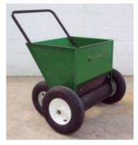
Tipping it back on two rear wheels allows you to move it about like a wheelbarrow, then tip it up on to all four wheels to begin spreading. Front end wheels power the spreading drum, mesh covered drum gives even spread of material. A sliding gate at front controls volume of output.
