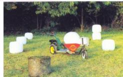
At harvest time a trailer can turn walking tractors into a transporter of produce from the garden, fruit from the orchard or hay from the far field. Hitched to a small compost spreader its ready to recycle organic matter.
