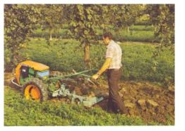
Primary tillage tools like reciprocating spaders Imats "rotary spaders" work a maximum of 24" wide digging respectively 6" and 10" deep.
