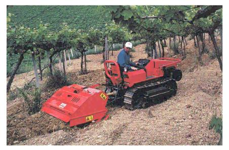
This is an ideal vineyard crawler for narrow plantings overall width under 40" yet 40 HP, enough for any task from spading to spraying. With 883 square inches of tread on ground you have low ground pressure and plenty of traction. A Cat I 3pt. and 540 PTO lets you operate all vineyard implements. Priced about the same as high quality wheel tractors of similar dimensions. It is impressive in every way.
