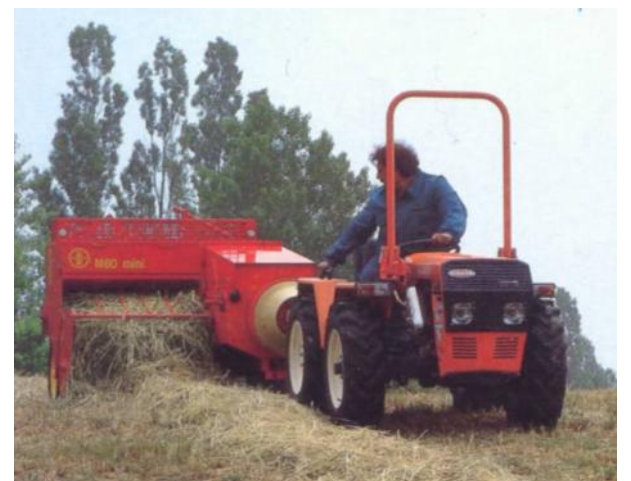
25 HP Trattorini powering a small square baler to produce 60+ pound bales of hay.
