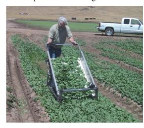
In its simplest form, machine is pushed by operator just as you would a push type lawn mower. Two bed-width rollers carry weight of machine with front roller controlling cutting height and rear roller supporting weight of machine and crop. Operator controls rate of advance to meet crop density and to insure
