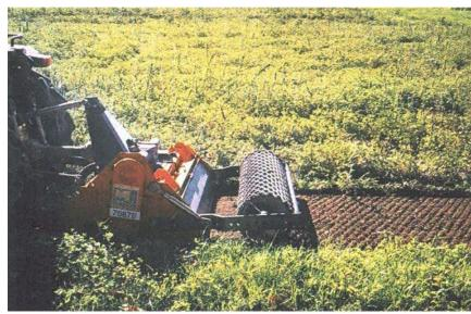
wide ready to plant bed is created. With the smallest of the Hydrostatic four wheel tractors a 33" bed is prepared in one pass. With a 30 HP tractor you could use a stone/burying tiller
