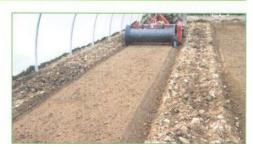
Now available, a small scale powered bed shaper/stoneburrier. This specialized tiller creates a raised finished bed and in the process sorts out small stones, twigs, roots and pieces of sod and burys them leaving several inches of clean soil on top of bed. This unit tills 39" wide creating a flat 22"wide bed top with tractors of 20 or more PTO HP.
