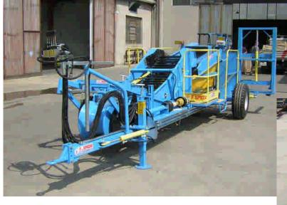
POTATO DIGGER SPECIAL - This machine has been designed to pick early and very delicate potatoes. The SPECIAL is a towed machine and the drawbar can be hydraulically controlled (opt.). The potato digger pickup consists of a system comprising adjustable tilt angle 3-blade share, swinging feeler roller for adjusting the digging depth, grass-cutting discs fitted on springs and
