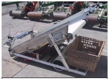
Side view shows adjusting screw to set front height adjustment, battery tray for one or more, large rear roller and tote platform.
