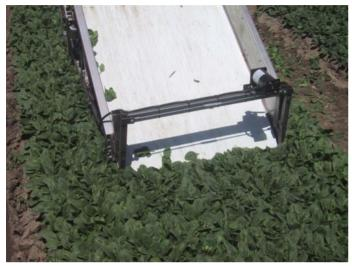
A separate electric motor with correct gear reductions permits food grade conveyor belt to catch crop at instant it is cut and to carry it up and into totes without being touched by anyone's hands, avoiding crushing and any possible contamination. A cutting width of 28" has been selected and the weight of machine and batteries have been minimized to allow machine to be hand pushed.
