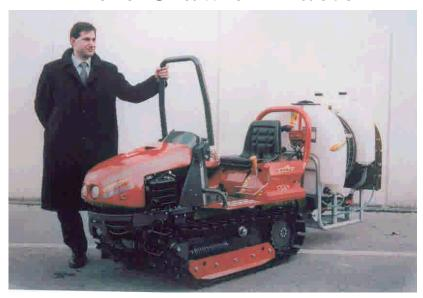
Fort Tractor Company now offers this small crawler with a 21 HP diesel. A 3pt and 540 PTO and narrow configuration makes it extremely attractive for high density vineyards. It is just 32" outside to outside and low to ground. Man in picture is 6ft 2" tall so you can see how compact this unit is and at \$20,000 it is a good value. Order now for early spring deliv-
