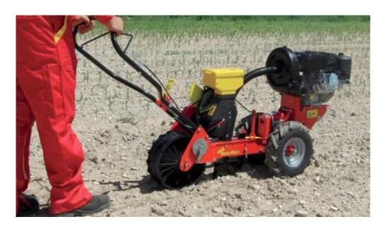
New seeder found at the EIMA show in Italy in November of 2012 and now in the USA. For \$4300.00 this self-powered vacuum seeder can plant any seed large or small without a tractor.
