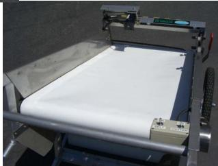
Standard unit uses wave edge stainless steel blade that moves from side to side. Band saw version uses similar but continuous cutting blade. Each cuts 28" wide swath.
