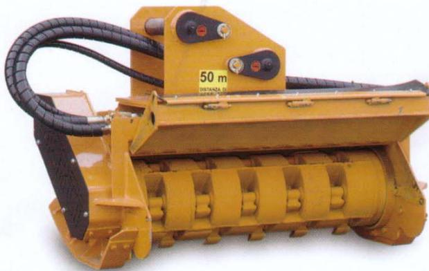
The rotor is equipped with double edge swinging hammers: being free to turn at 360°, the hammers prevent the rotor from being roughly hit and allow the machine to work on uneven terrains and/or rocky conditions.
