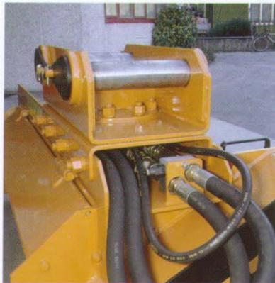
The Anti-cavitation system safeguards the hydraulic motor against the cavitation effect which is created when the rotation speed is strongly reduced or stopped.
