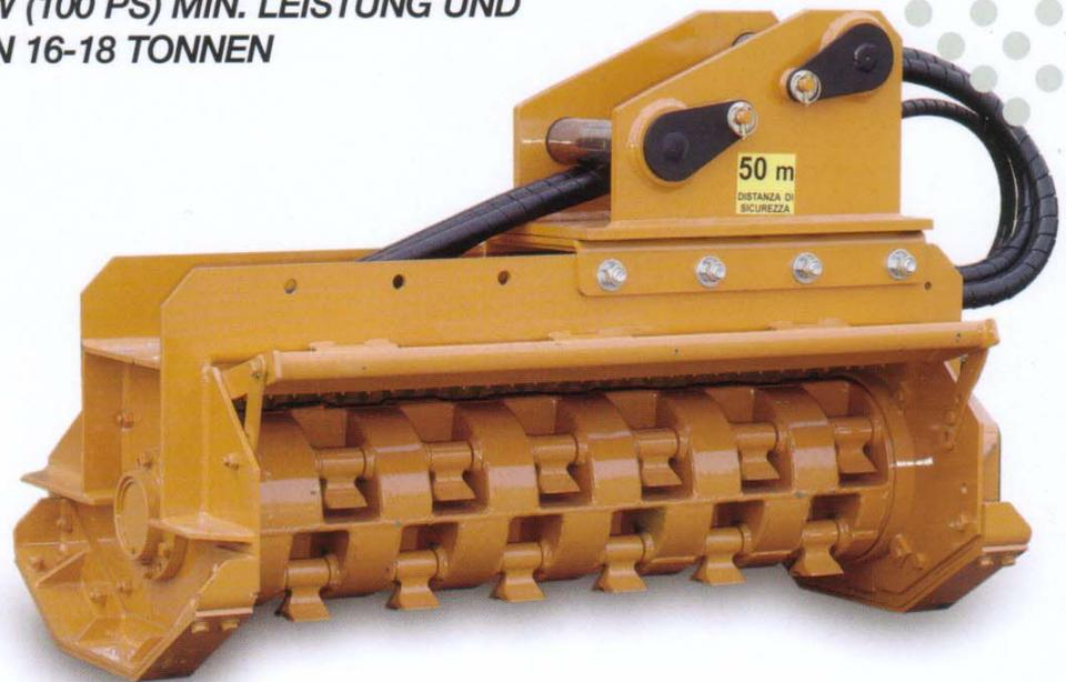
Reliable and sturdy machine, it can shatter grass, brush, branches and trunks up to a diameter of 15 cm (6"), particularly in the clearance and maintenance of waterways, banks, ditches, power lines, railways and for the clearance of derelict areas and fire breaking lines. The rotor is equipped with double edge swinging hammers: being free to turn at 360°, the hammers prevent the rotor from being roughly hit and allow the machine to work on uneven terrains and/or rocky conditions.
