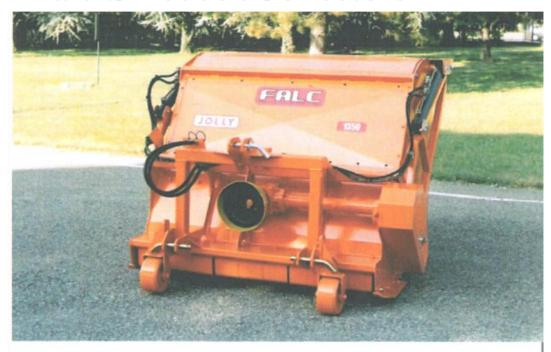
Falc now offers a wide range of shredders that collect cut material so it can be removed from field. The elevated dump system allows material to be put onto truck bed or trailer. This makes it easy to remove prunings that might harbor pests and/or material for composting.
