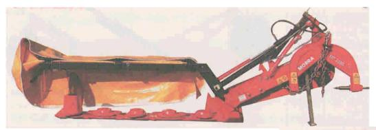
The disc mower is ideal for making hay but also handles brambles better than syclebar mowers. Cuts clean, following ground contours and does not plug up. Each disc is mounted on its own ball bearing supported spindle and driven by adjacent spur gear, also ball bearing supported, giving smooth efficient power transfer. A (4) disc model cutting 63" swath, suitable for 30 HP, costs \$4,000 delivered. Other larger models up to 9 ft. cut are also available.
