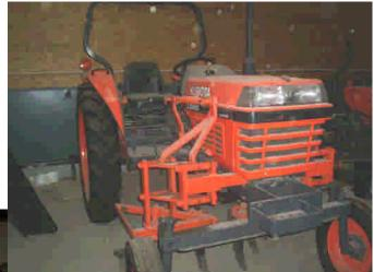
Actually they have extended front and rear axles to the right, adjusted tractor controls and fabricated a system to raise and lower cultivator assembly.
