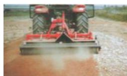
Stone burying/bed making Tiller
