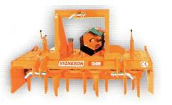
Ideal way to break clods left by plowing, discing or spading. By stirring instead of turning, the power harrow breaks up clods and leaves the ground perfectly flat. Ideal for preparing a smooth seed bed.
