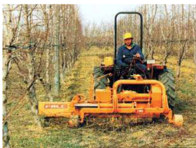
Falc Sonar Shredder is a heavy duty flail mower that offsets 16 inches automatically when sensor wand touches tree. All hydraulics are self contained and unit can be used either front or rear mounted. Shown on Antonio Carraro Bidirectional tractor.
