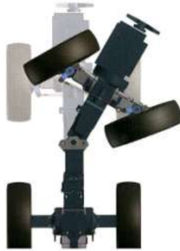
Dual Steer is unique steering system that combines conventional front axle steering with an articulated chassis to give 70 degree turns.
