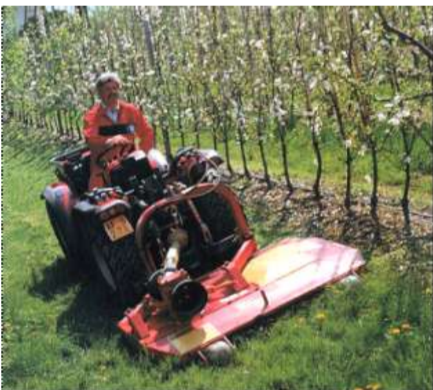
Antonio Carraro SRX 8400 articulated 63 HP bidirectional tractor shown with a rotary mower with manually controlled parallelogram hydraulic offset.
