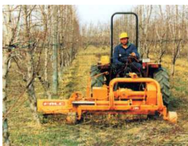
Falc Sonar Shredder is a heavy duty flail mower that offsets 16 inches automatically when sensor wand touches tree. All hydraulics are self contained and unit can be used either front or rear mounted. Shown on Antonio Carraro Bidirectional tractor.
