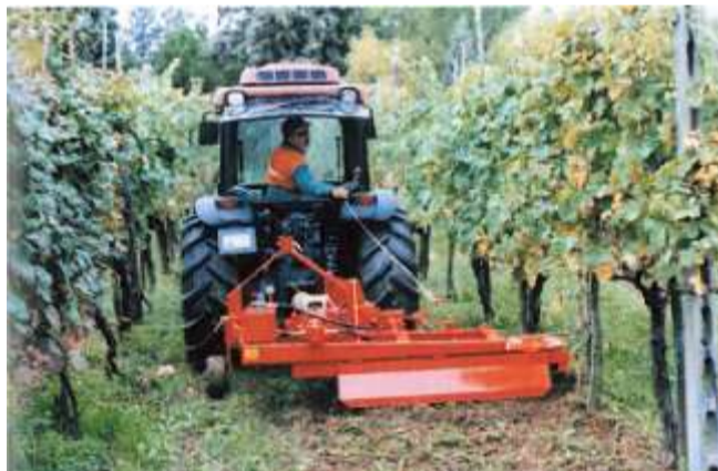
Rinieri EP works like the EL but works deeper and wider.
