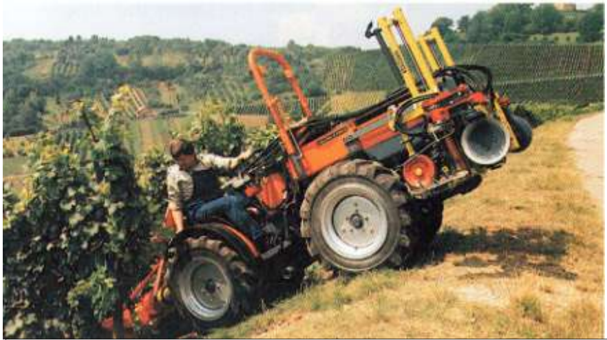
Clemens hoe mounted on front of Goldoni tractor leaves 3 pt. free to run mower simultaneously.
