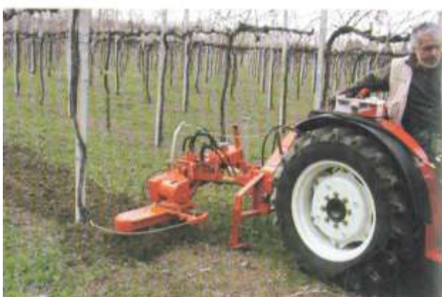
Rinieri EL140 tilling berm area. Note sensor has finer sensitive touch.
