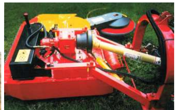
Fischer SL90—Front mount rotary mower with sensor controlled rotary outrigger.
