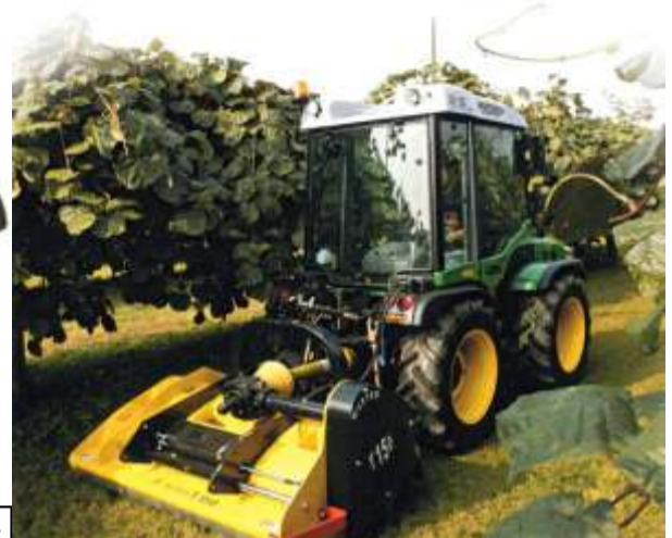
Muster mowers have 2 flail rotors to reduce vegetation to fine mulch and can offset to work under overhanging plants and around obstacles. The Muster can be used in front or behind tractor.
