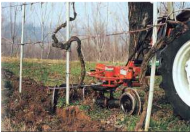
Rinieri powered berm disc cutting deep.
