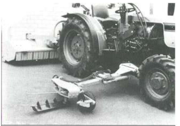
Side mounting of Clemens hoe version that reaches under wide canopy to till berm.
