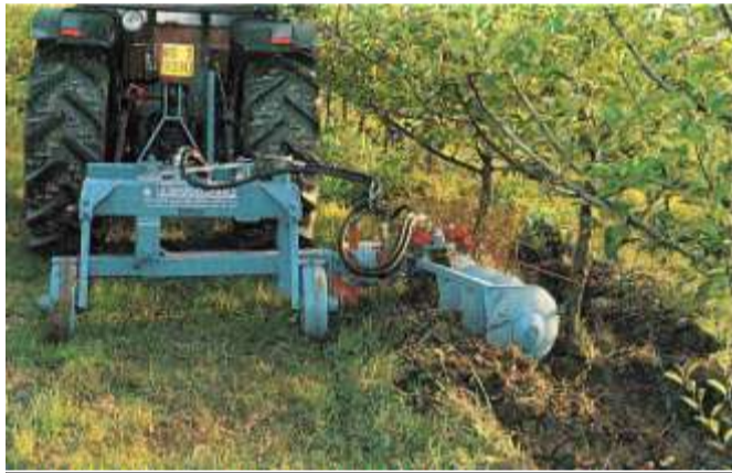
A.Spedo TPE powered berm disc showing aggressive weed control
