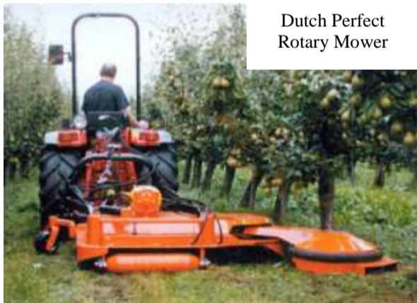
Note low profile with rounded surfaces of Dutch made Perfect Rotary Mower with outrigger.
