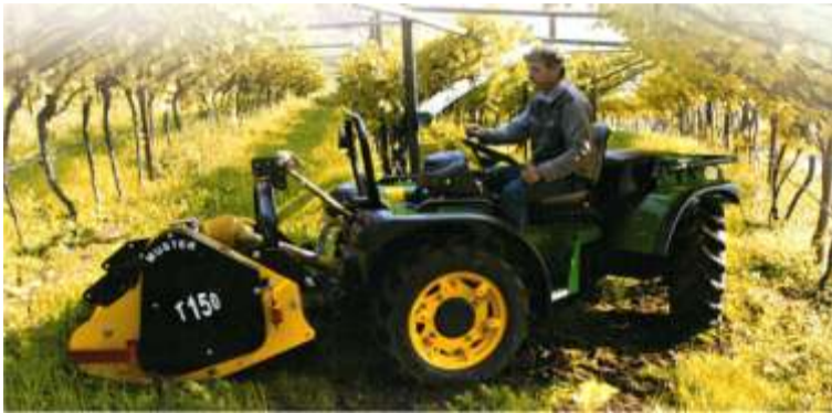
Ferrari Dual Steer Vega 75 (64 HP) shown with BCS Muster double rotor flail mower, weight of tractor and mower equally divided over four equal size drive wheels.
