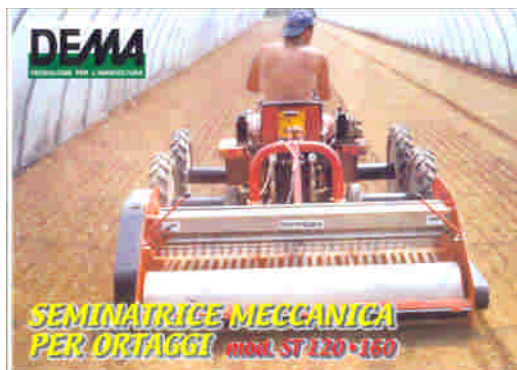
26 HP Carraro tractor with wheel spacers to span 60". Shown with precision salad mix seeder. Seeders can be had 39" and 48" wide.
