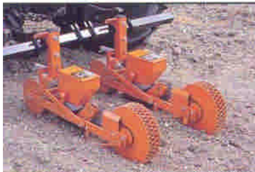
Even smallest tractor can operate precision belt planters each metering unit can put down 1 to 3 lines of seed. Precise spacing minimal doubles mean less thinning and easier tillage.
