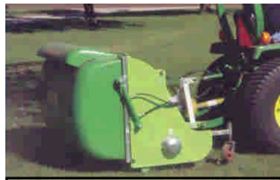
48" wide flail mower with Collector. Mow strips between beds and collect material for compost.
