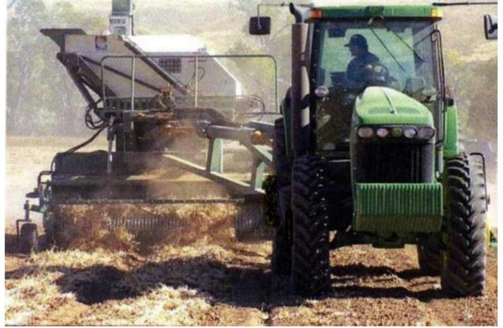
When bean vegetation is sufficiently dry the large scale grower would use a special pull type combine to pick up windrowed plants and thresh out beans as it travels along windrow. There is no economically viable small version of this machine.
