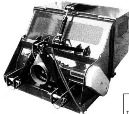
Still another labor saving method of harvesting is to use a mower/collector to pick up windrowed crop. Some bean breakage will result from high speed and aggressiveness of flail blades, but broken beans can be used at home and/or as protein supplement for livestock. The mower/collectors come in many sizes and can cost less than balers.
