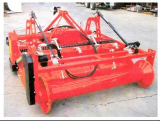
Pictured here is an 80 inch wide Massano tiller that creates a 64 inch bed top that is firmed and finally defined by a hydraulically driven rear roller. Note individual coil springs of the tines that make up the comb behind the rotor.
