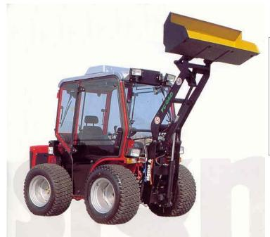
This same model loader was originally designed specifically for Antonio Carraro's hydrostatic tractor model Sp 4400 and HST 4400 (38 HP). Loader has a hydraulic jack stand so that mounting and demounting loader is easily done by operators without strain and requires no tools.
