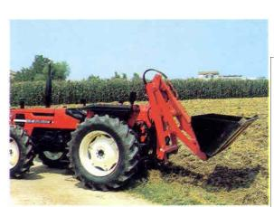
Still another rear loader manufacturer uses the tractors 3 pt arms to support the entire loader. A hydraulic top link allows loader mast to be tilted to bring load in closer to tractor. Nemag makes 6 models to fit 20 to 130 HP tractors.
