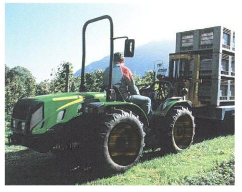
If you need 60 to 90 HP Ferrari offers the Thor and Vega series with the same iso-diametric driving wheels i.e. equal size with equal distribution of weight and traction. These larger models also come in Articulated and front steer versions and can be had mono directional or with bidirectional
