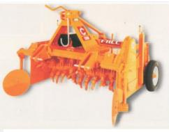
clods and gives a good soil finish without glazing the subsoil or over working top soil as conventional rototillers would.
