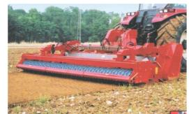
tines. Soil, fine, free of debris, pass through while stones, root clumps and other debris fall to the bottom of the cut and are buried by clean soil. Mesh roller firms soil and leaves it uniformly flat.
