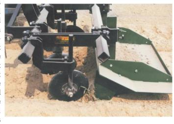
of the shaper to give a uniformly smooth growing areas. Small discs or plow shares set at angles help direct soil flow.
