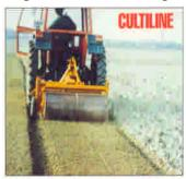
The rotoking also can be equipped with bed defining side plates, depth control wheels and a smooth rear roller to create a finished seed bed in a single pass. This configuration is called the FALC Cultiline. The larger model rotokings can be equipped with rear rollers and rear 3 pts to permit a seeder to be mounted so it can be deployed in the same pass as the rotoking eliminating one more trip over the field.
