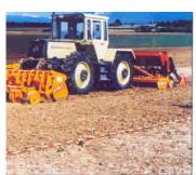
When very large acreages are to be worked two remarkable machines are worth considering because they accomplish their work at dramatically higher speeds than those referred to above. The first of these is the Falcland; in effect this is a PTO driven rotary chisel that opens up soil 17.5 inches deep while traveling up to 3.5 miles per hour using about 150 HP.
