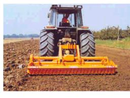
Another primary tillage tool worth considering is the Falc Rotoking. This is a rotary type tiller but differs from a rototiller in the design of it's soil opening components. Instead of "C" or "L" shaped tines that cleave and then "trowel" the soil overworking the top portion and smearing the underside of the cut, the rotoking has a rotor equipped
