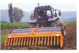
The rotoking is also equipped with a (4) speed gearbox allowing you to adjust rotor speed to soil conditions so you can prevent overworking soil and avoid destruction of soil tilth and the resulting crusting of soil surface. In addition to being used for primary tillage the Rotoking is effective as a secondary tillage tool to perfect a seedbed after chiseling, plowing, stubble discing or spading, whenever clod size must be reduced to permit correct seed placement and coverage.
