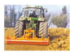
The Power Harrow is a tool designed for secondary tillage and thus used to reduce clod size from that left by primary tillage operation and to prepare a finished seed bed. The power harrow uses tines turning on vertical axis to create a stirring action and does not turn over the soil. These pairs of tines over-
