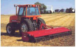
The second of the higher speed tools is known as a Dynadrive. This unusual machine is ground powered rather than PTO driven. Two rotors with "spoon like" tines churn up to the soil incorporating grass or grain stubble. The front rotor drives the rear rotor at a different speed to tear up roots and leave a
