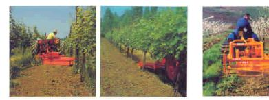
A somewhat more recent development is the offsetting power harrow that uses tines rotating on vertical axis. As with the rototiller these can be designed to do narrow bands or wide enough to do much of the row centers in each pass.
