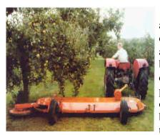
In these the outrigger is usually a rotary mower driven by a belt or hydraulic motor and mounted on an arm that is spring loaded. A rubber bumper on the blade guard comes in contact with the trunk of the crop plant causing the outrigger to move out and around the plant. Once the blade guard, that protected plant trunk from being damaged, is no
