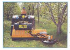
A more sophisticated version of the outrigger system uses a hydraulic cylinder to deploy the outrigger and uses a wand to contact crop plant and control mower movement. The wand opens and closes a hydraulic valve to control action and impact on crop is extremely light.
