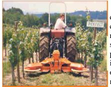
The first group are mowers designed to keep compatible covers crops clipped short to deny weed varieties a chance establishing themselves in significant numbers, and to prevent them from maturing and going to seed. The simplest form is an outrigger mounted on the side of a mower used to mow the centers.
