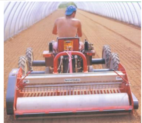
Note seed pockets on rotor
