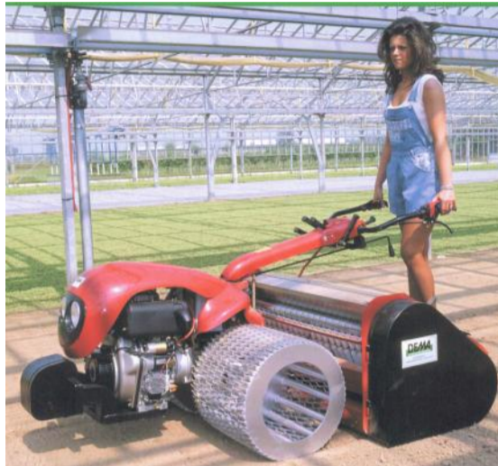
Note seed pockets on rotor
